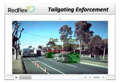
The non-intrusive technology used (exclusive to Reflex) is capable of, from a single pole location, determine multiple vehicle movements and in the example above the distance relative to each other dynamically and without post processing data and information. This allows for on the spot detection, evaluation and information capturing to ensure comprehensive data is delivered to the processing facility for enforcement.
